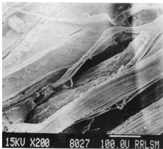
Figure 5 (a) SEM photograph showing longitudinal orientation of fibers in SBR composite (mix C). (b) SEM photograph showing transverse orientation of fibers in untreated SBR composite (mix C).
